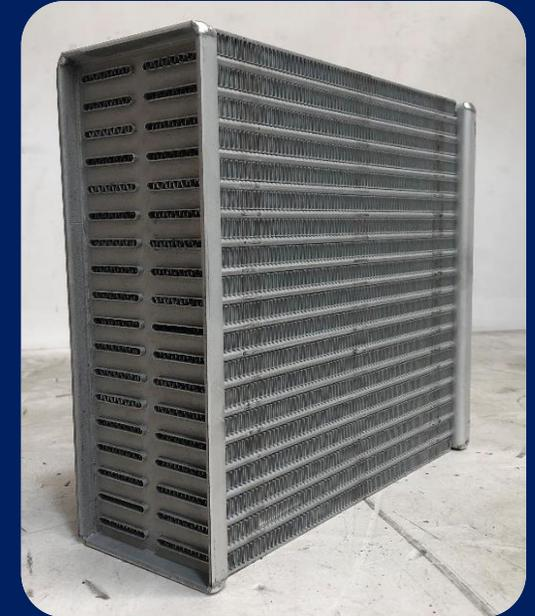
*Watercooler welded tubes*
